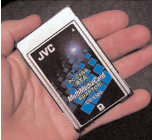
Figure 27.3 PCMCIA cards are excellent storage devices for digital images and can easily be attached to all current notebook computers and to desktop computers with an appropriate slot.
