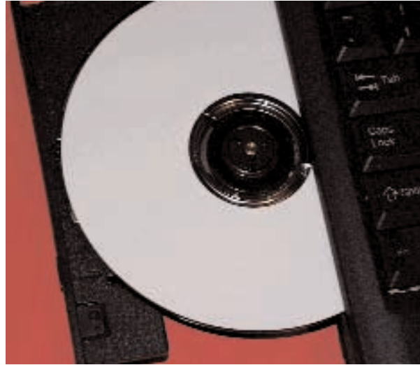
Figure 27.8 A removable CD recorder with a notebook computer is the author's choice for mobile data backup.
