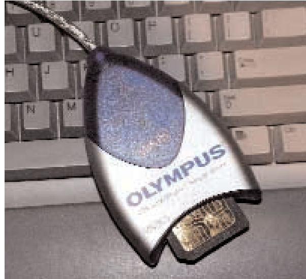
Figure 27.6 USB card-readers are a great and portable alternative for reading SmartMedia cards and other types of digital camera storage cards. Most new computers have USB ports which enable the use of this type of card-reader.
